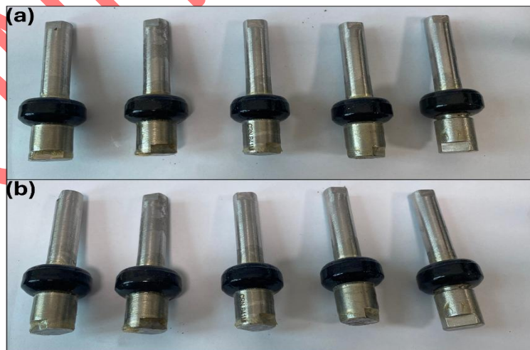
Figure 3. Images of five black powder charges coated with adhesive sample M3-3: (a) before and (b) after 10 thermal-humidity cycles
